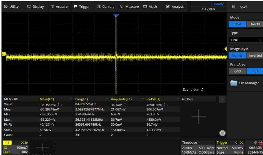
Figure 2.6: Potential event recorded on the test detector. This was in the two GEM setup with 1050 V total,
