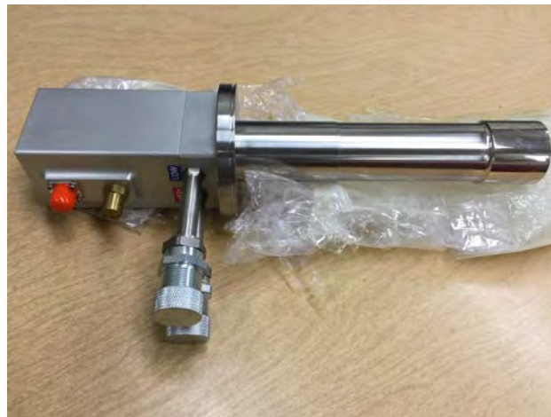
Figure 2 shows the AL60 cold head. To make a fully vacuum-jacketed condenser would require two seals on the cold head. The flair at the end of the cold head prevents one of the seals from being on the stem (the cold head has fit into the condenser). Because the stem being an unsuitable sealing area, the inner seal must be on the flange at the center. Again as with the stem, if the flange is to be the inner seal, then it must fit through the outer seal, which would need to be on the square part of the instrumentation region, which is not feasible.
