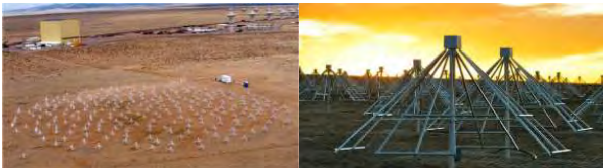
Figure (5): The first station of the Long Wavelength Array (LWA1) and a close-up individual stand consisting of 2 orthogonal dipole elements angled down by 45 degrees to improve sensitivity at mid elevation angles [61].
