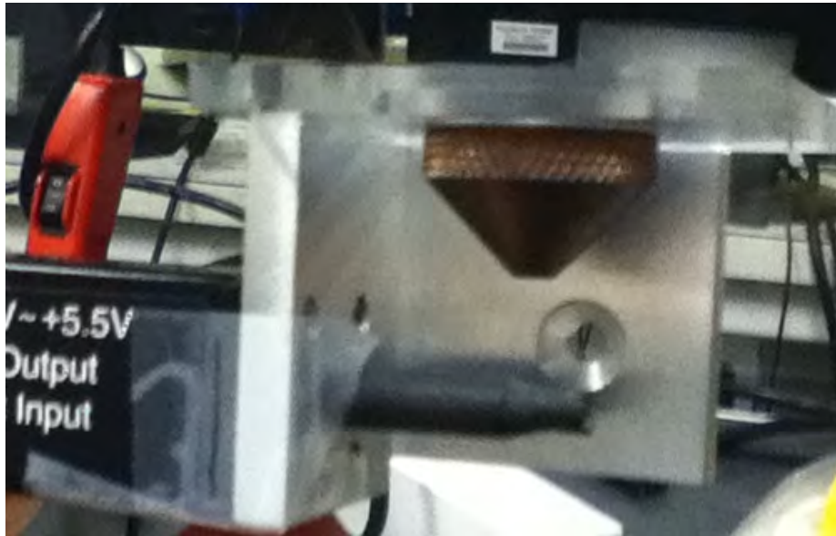
Figure 3.4: The PMT-scintillator assembly is shown. The PMT is located at the left, where it is connected to the housing of the collimator, top center, and the scintillator, center. The radiation source, Sr-90, is placed atop the collimator, which directs the beam of charged particles to the scintillator, after they have passed through the diamond.
