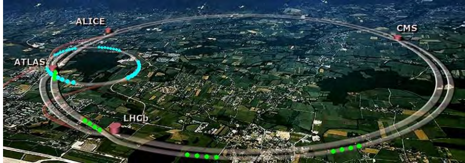
Figure 1.1: An aerial photograph of the location of the LHC on the Franco-Swiss boarder overlaid with a map of the LHC and its primary detectors, ALICE, ATLAS, CMS and the LHCb. The LHC includes a tunnel 27 km in circumference at a depth of up to 175 meters below the surface.
