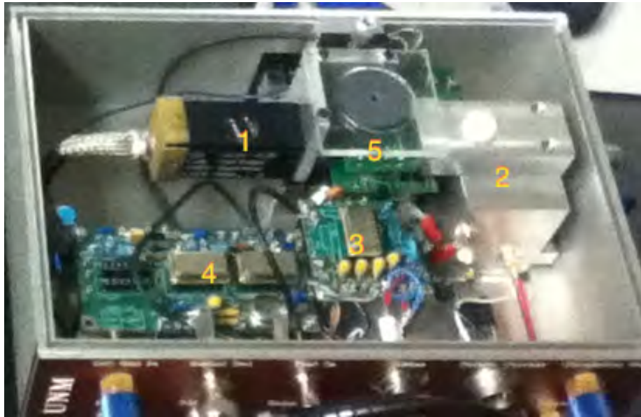
Figure 3.3: The interior of the preamplifier box showing the location of the components. The main components are: 1. the PMT-scintillator-collimator assembly 2. the airflow block that rests atop of the Peltier temperature control, 3. PC250 board and 4. PC275 board. The diamond samples are place under the collimator at 5.
