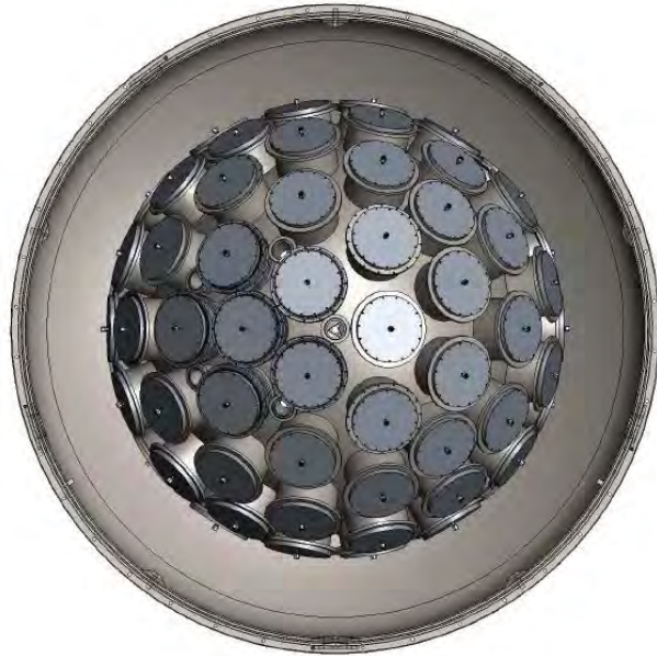
Figure 7: A cut away view of the MiniCLEAN detector's inner vessel and the surrounding outer vessel. The top hats of the 92 optical cassettes along with the calibration ports are visible.
