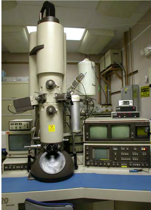
Figure 4: Our 200 keV Philips CM20 Transmission Electron Microscope.
