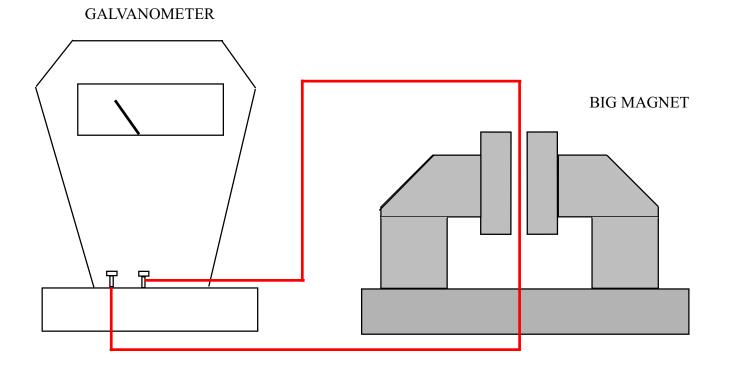
REMOVE WRISTWATCH WHEN USING BIG MAGNET. MAGNET IS VERY HEAVY. PICK UP WITH CARE. CONNECT SINGLE WIRE FROM GALVANOMETER/VOLTMETER CON-NECTION TO GALVANOMETER CONNECTION. LOOP WIRE OVER MAGNET THROUGH SPACE BETWEEN PLATES. MOVING WIRE BETWEEN POLES OF MAGNET CAUSES DEFLECTION OF GALVANOMETER NEEDLE. REVERSING WIRE CAUSES NEEDLE TO BE DEFLECTED IN OPPOSITE DIRECTION.
