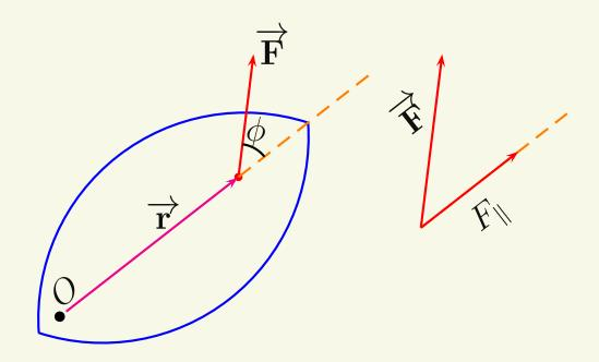
The direction of the force also determines the torque. When  $\overrightarrow{\mathbf{F}}$  is not perpendicular to the lever arm  $(\overrightarrow{\mathbf{r}})$ , only the component of  $\overrightarrow{\mathbf{F}}$  which is perpendicular to  $\overrightarrow{\mathbf{r}}$  causes torque.
