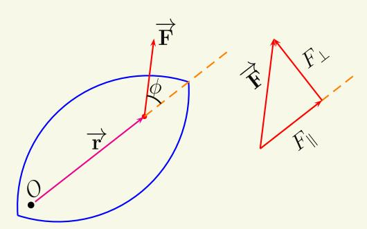
$F_{\parallel}$  - component parallel to  $\overrightarrow{\mathbf{r}}$  - causes no torque
