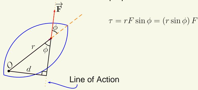
The calculation of torque can be simplified in some cases by the use of the perpendicular distance.
