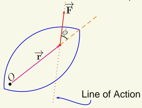
The calculation of torque can be simplified in some cases by the use of the perpendicular distance.
