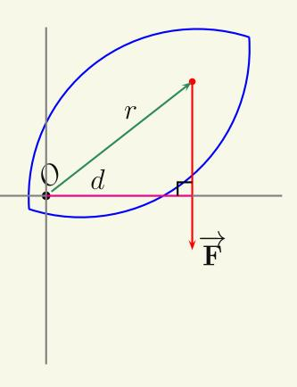
The perpendicular distance is particularly useful in finding the torque exerted by vertical forces.
