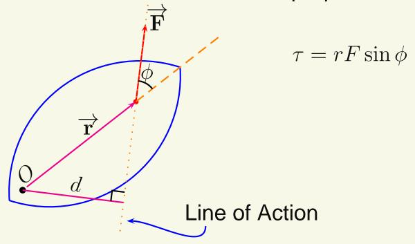
The calculation of torque can be simplified in some cases by the use of the perpendicular distance.
