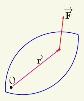
The direction of the force also determines the torque. When  $\overrightarrow{\mathbf{F}}$  is not perpendicular to the lever arm  $(\overrightarrow{\mathbf{r}})$ , only the component of  $\overrightarrow{\mathbf{F}}$  which is perpendicular to  $\overrightarrow{\mathbf{r}}$  causes torque.
