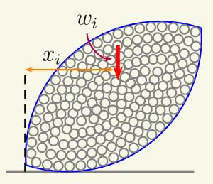
Real objects consist of many particles. When experiencing a gravitational torque, each individual particle experiences a torque.
