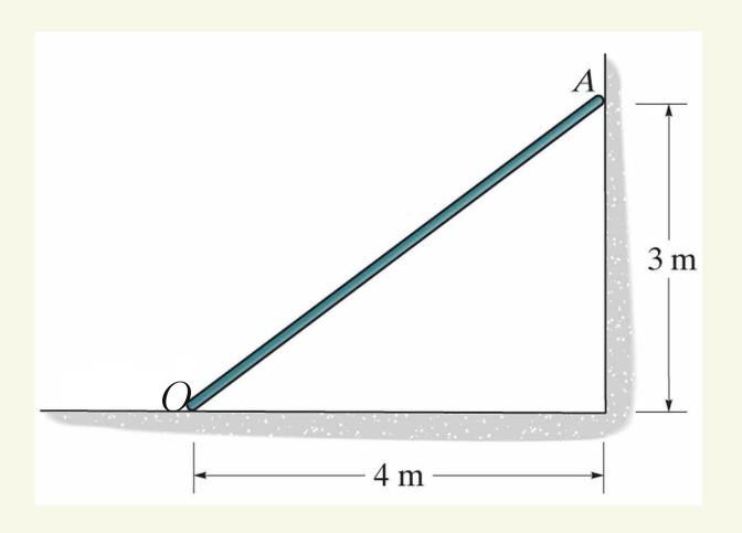
A 300-N uniform bar is leaning against a wall as shown. What is the gravitational torque magnitude about the point O?
