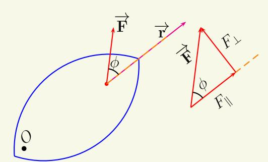
$F_{\parallel}$  - component parallel to  $\overrightarrow{\mathbf{r}}$  - causes no torque
