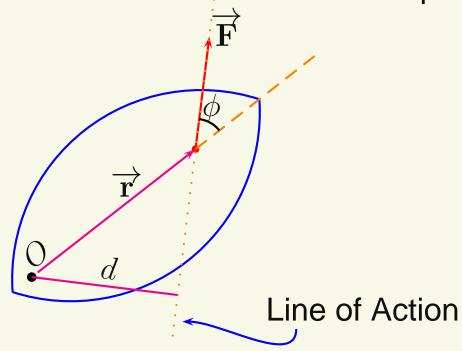
The calculation of torque can be simplified in some cases by the use of the perpendicular distance.
