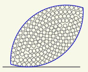
Real objects consist of many particles. When experiencing a gravitational torque, each individual particle experiences a torque.
