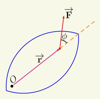
The direction of the force also determines the torque. When  $\overrightarrow{\mathbf{F}}$  is not perpendicular to the lever arm  $(\overrightarrow{\mathbf{r}})$ , only the component of  $\overrightarrow{\mathbf{F}}$  which is perpendicular to  $\overrightarrow{\mathbf{r}}$  causes torque.
