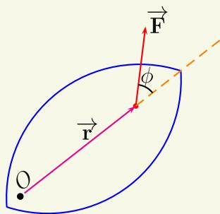
The calculation of torque can be simplified in some cases by the use of the perpendicular distance.
