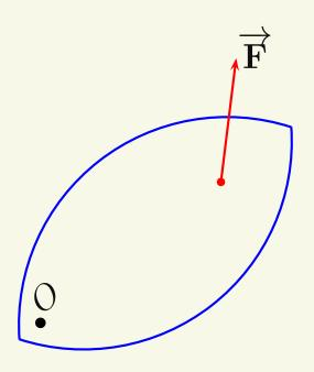
The direction of the force also determines the torque. When  $\overrightarrow{\mathbf{F}}$  is not perpendicular to the lever arm  $(\overrightarrow{\mathbf{r}})$ , only the component of  $\overrightarrow{\mathbf{F}}$  which is perpendicular to  $\overrightarrow{\mathbf{r}}$  causes torque.
