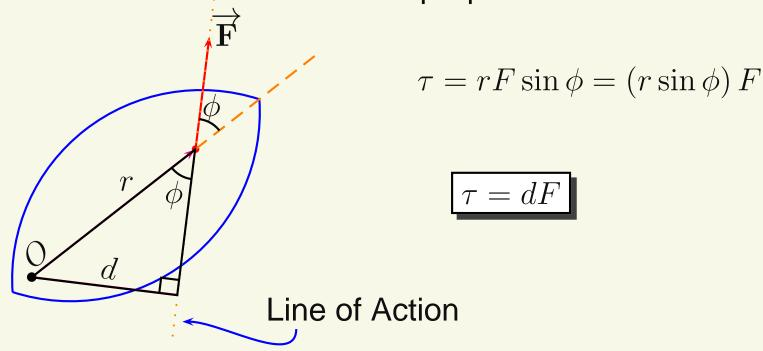
The perpendicular distance is particularly useful in finding the torque exerted by vertical forces.
