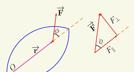
$F_{\parallel}$  - component parallel to  $\overrightarrow{\mathbf{r}}$  - causes no torque
