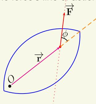
The calculation of torque can be simplified in some cases by the use of the perpendicular distance.
