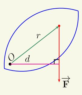
The perpendicular distance is particularly useful in finding the torque exerted by vertical forces.
