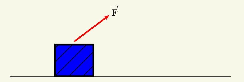
Only the component of the force parallel to the displacement does work.
