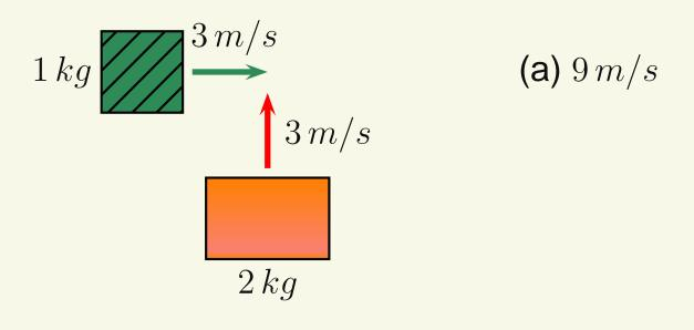
A block with  $M_A=1\,kg$  and velocity  $3\,m/s$  to the right has a perfectly inelastic collision with  $M_B=2\,kg$  that has velocity  $3\,m/s$  up. How fast must the masses be going the instant after their collision?
