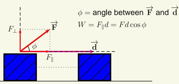
Only the component of the force parallel to the displacement does
