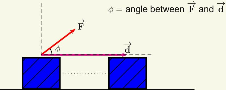
Only the component of the force parallel to the displacement does
