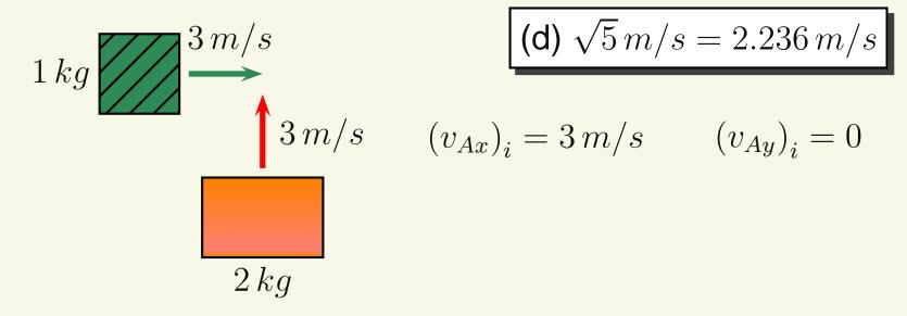
A block with  $M_A=1\,kg$  and velocity  $3\,m/s$  to the right has a perfectly inelastic collision with  $M_B=2\,kg$  that has velocity  $3\,m/s$  up. How fast must the masses be going the instant after their collision?
