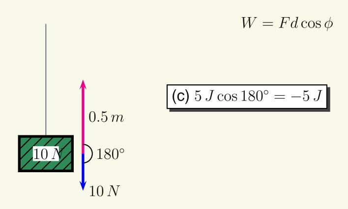
A  $10\,N$  block is pulled  $0.5\,m$  upwards with constant speed by a massless rope. How much work is done by gravity?
