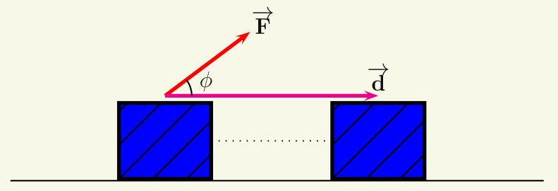
Only the component of the force parallel to the displacement does
