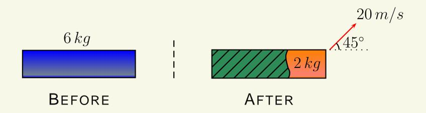
A 6 kg box-shaped firecracker explodes into two unequal pieces. If the first piece of mass 2 kg has velocity 20 m/s at  $45^{\circ}$ , what speed and direction must the other piece have?
