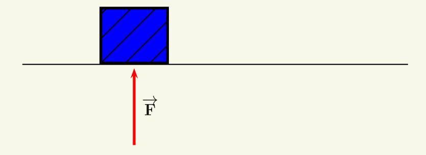
A force perpendicular to the displacement does no work.
