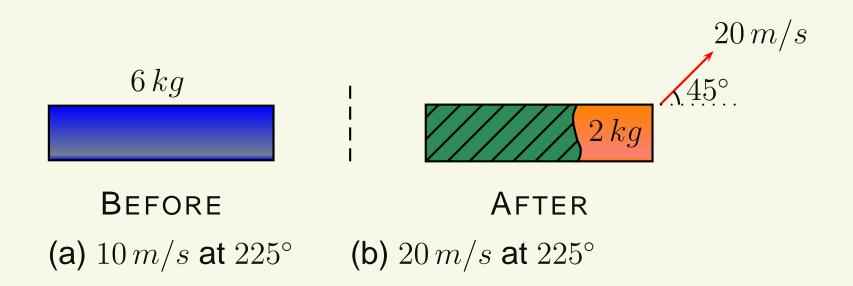
A 6 kg box-shaped firecracker explodes into two unequal pieces. If the first piece of mass 2 kg has velocity 20 m/s at  $45^{\circ}$ , what speed and direction must the other piece have?
