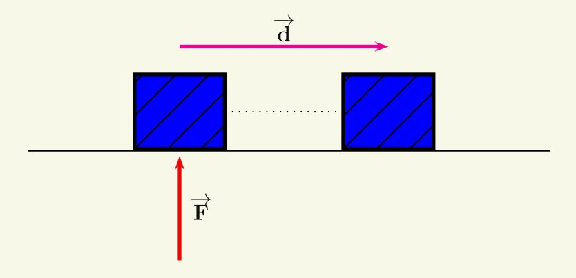
A force perpendicular to the displacement does no work.
