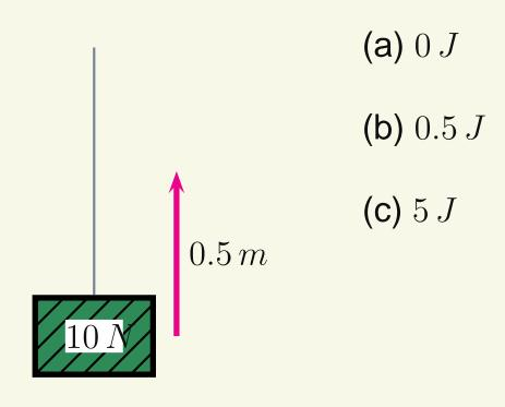
A  $10\,N$  block is pulled  $0.5\,m$  upwards with constant speed by a massless rope. How much work is done by the tension force?
