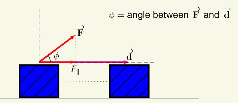
Only the component of the force parallel to the displacement does
