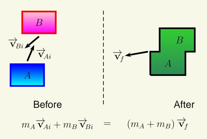
Component Form:  $m_A (v_{Ax})_i + m_B (v_{Bx})_i = (m_A + m_B) (v_x)_f$  $m_A (v_{Ay})_i + m_B (v_{By})_i = (m_A + m_B) (v_y)_f$
