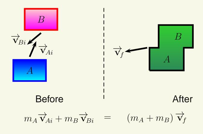
When the colliding objects stick together, the collision is called completely inelastic.
