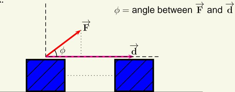
Only the component of the force parallel to the displacement does
