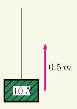
A  $10\,N$  block is pulled  $0.5\,m$  upwards with constant speed by a massless rope. How much work is done by gravity?
