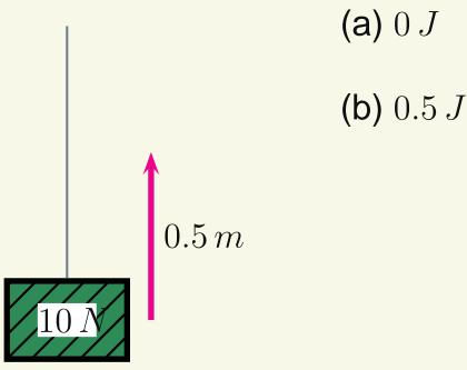
A  $10\,N$  block is pulled  $0.5\,m$  upwards with constant speed by a massless rope. How much work is done by the tension force?
