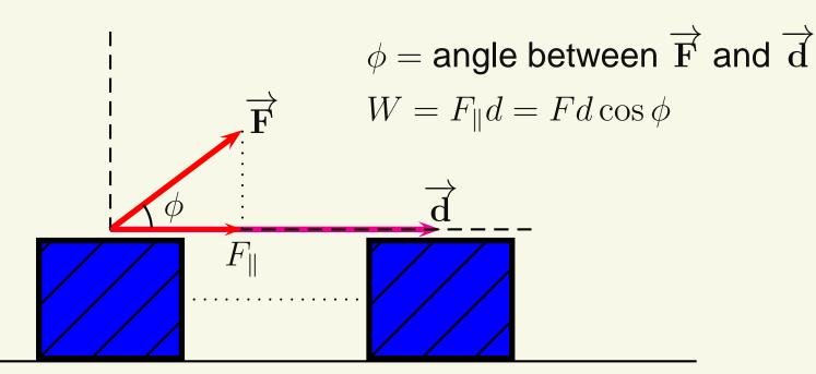
Only the component of the force parallel to the displacement does
