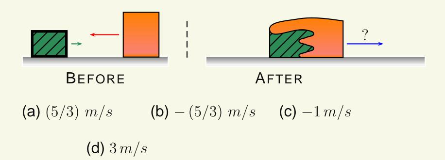
A 1-kg mass sliding to the right with speed 1 m/s on a frictionless floor collides with a 2-kg mass going to the left at 2 m/s. If the masses stick to each other, how fast is the combo going after?
