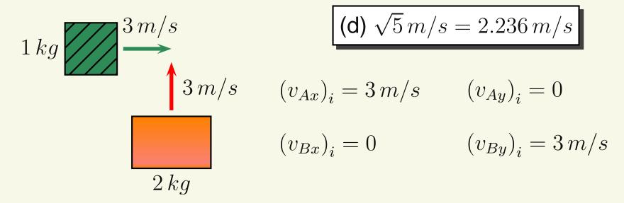
A block with  $M_A=1\,kg$  and velocity  $3\,m/s$  to the right has a perfectly inelastic collision with  $M_B=2\,kg$  that has velocity  $3\,m/s$  up. How fast must the masses be going the instant after their collision?
