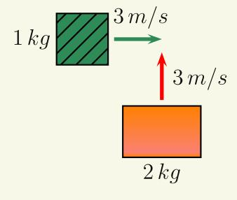
A block with  $M_A=1\,kg$  and velocity  $3\,m/s$  to the right has a perfectly inelastic collision with  $M_B=2\,kg$  that has velocity  $3\,m/s$  up. How fast must the masses be going the instant after their collision?
