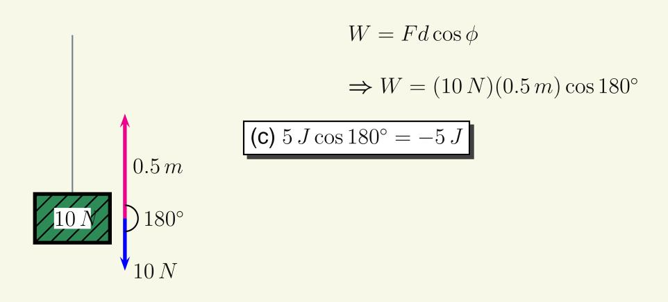
A  $10\,N$  block is pulled  $0.5\,m$  upwards with constant speed by a massless rope. How much work is done by gravity?
