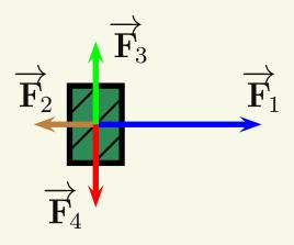
A box is subjected to the four forces shown. Which of the following correctly shows the net force  $\sum \overrightarrow{F}$  acting on the box?
