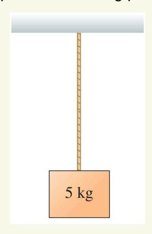
A 5 kg mass is hung from the ceiling using a "massless" rope. What is the magnitude of the tension force exerted by the rope on the mass? **Hint:** A 5 kg mass has a weight of 49 N on earth where this problem is taking place.
