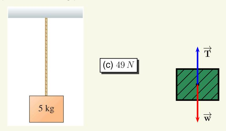
A 5 kg mass is hung from the ceiling using a "massless" rope. What is the magnitude of the tension force exerted by the rope on the mass? **Hint:** A 5 kg mass has a weight of 49 N on earth where this problem is taking place.
