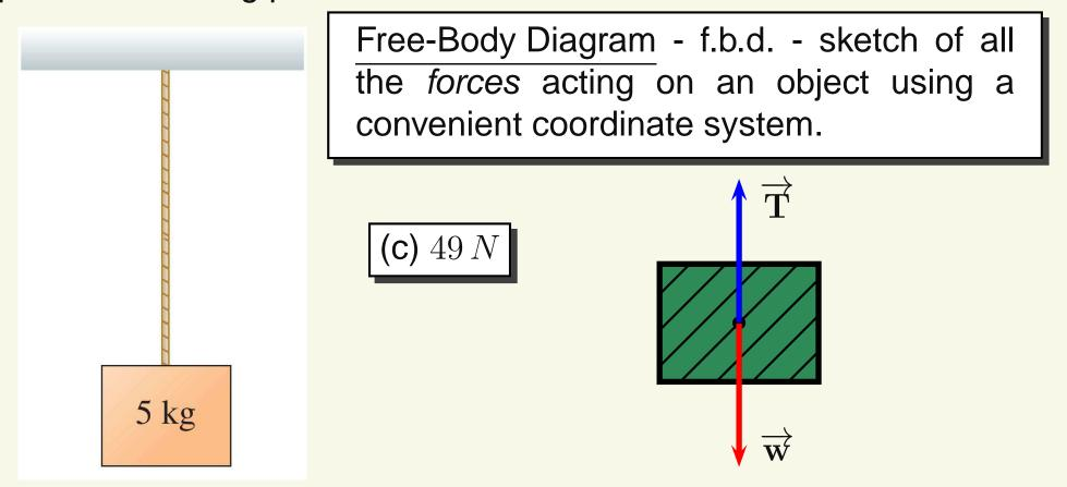
A 5 kg mass is hung from the ceiling using a "massless" rope. What is the magnitude of the tension force exerted by the rope on the mass? **Hint:** A 5 kg mass has a weight of 49 N on earth where this problem is taking place.
