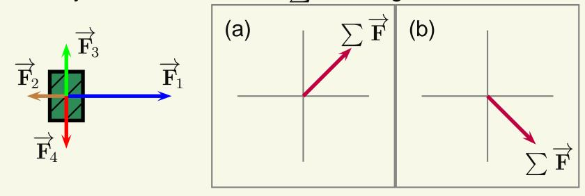
A box is subjected to the four forces shown. Which of the following correctly shows the net force  $\sum \overrightarrow{F}$  acting on the box?
