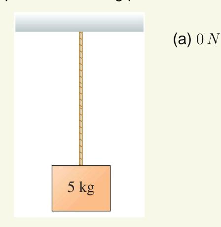
A 5 kg mass is hung from the ceiling using a "massless" rope. What is the magnitude of the tension force exerted by the rope on the mass? **Hint:** A 5 kg mass has a weight of 49 N on earth where this problem is taking place.
