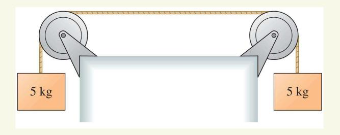
Two 5 kg masses are connected to each over pulleys using a rope. What is the tension force that the rope exerts on the right-hand mass if they are both at rest?
