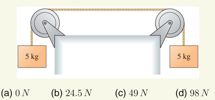
Two 5 kg masses are connected to each over pulleys using a rope. What is the tension force that the rope exerts on the right-hand mass if they are both at rest?
