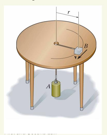
Block B is circling around a rough table while connected to a rope that passes through a hole in the center of the table down to cylinder A. Which of the following forces do we NOT identify as acting on the block B?
