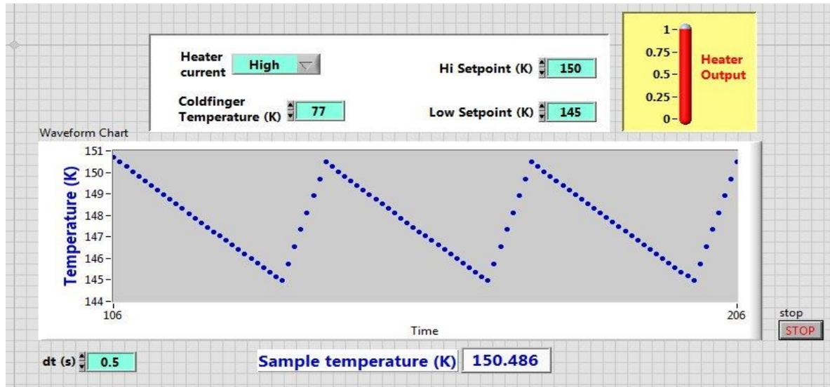
In the next lab, this assigned VI will be interfaced to the Elvis board to control the temperature of a tiny “oven”.
