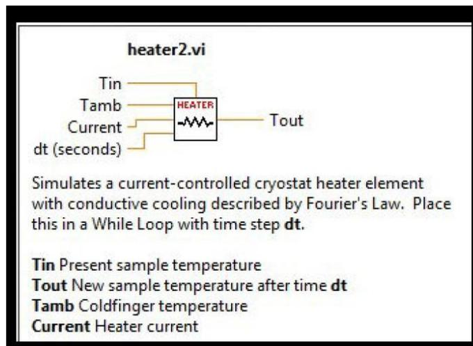
**Tamb** is the reservoir temperature, which is 77K for liquid nitrogen. **Tin** and **Tout** are the input and output temperatures, respectively; wire these to the corresponding terminals of a shift-register. The time **dt** is also the Wait time of the While Loop (note that the subVI requires *s* not *ms*).
