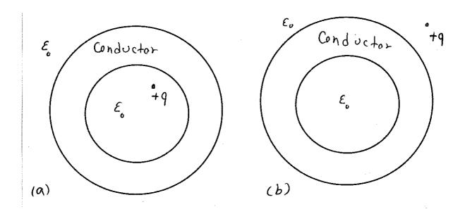
3— A capacitor consists of two concentric spherical surfaces of radii a, b. Part of the space between these surfaces is filled with dielectric material of permittivity  $\epsilon$  as shown in the figure. What is the capacitance?
