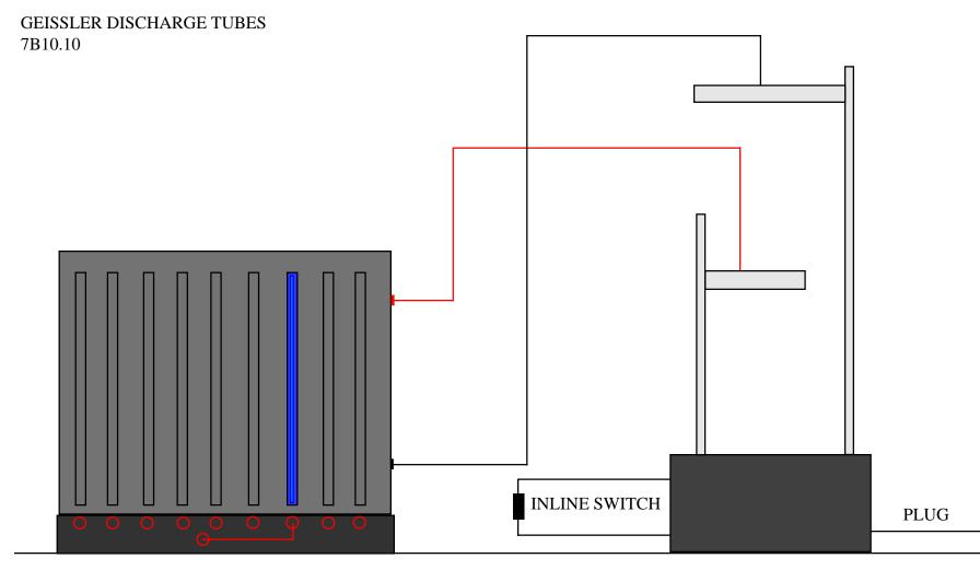
SEVERE SHOCK HAZARD! TURN POWER OFF AT INLINE SWITCH BEFORE CHANGING TUBE WIRING.
