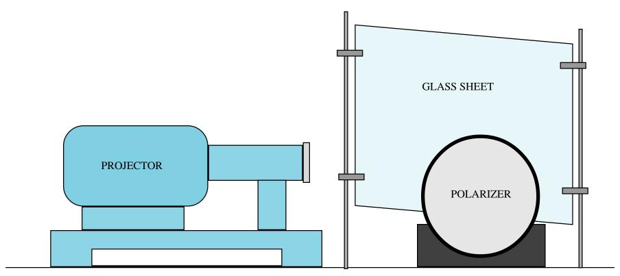
SET UP ON ONE CART. SECURE GLASS SHEET FIRMLY. USE ONLY ONE POLARZER.
