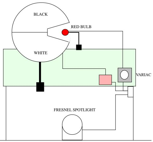
THE DISK, AS SHOWN, IS ROTATED AT 2 - 3 RPS BY THE DIRECT DRIVE BODINE MOTOR WITH SPEED CONTROL.
