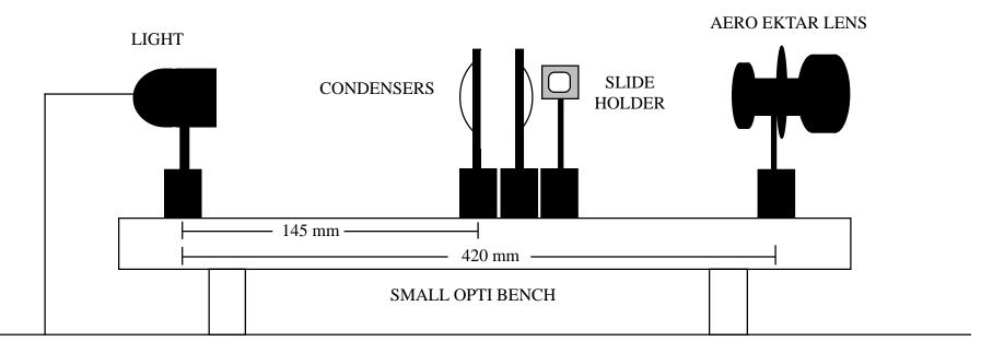
SET UP ON SMALL OPTI - BENCH. USE AERO EKTAR LENS AND SMALL LIGHT SOURCE.
