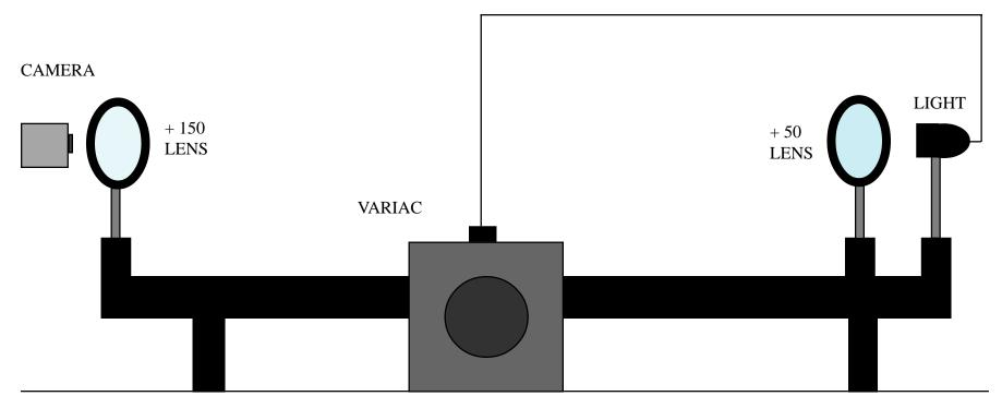
USE VARIAC TO REGULATE POWER TO LAMP. INCREASE POWER TO LAMP UNTIL FILAMENT IS BARELY VISIBLE.
