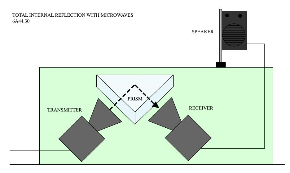
IF RECEIVER IS MOVED TO DIRECTLY ACROSS FROM THE TRANSMITTER THERE IS NO PICK UP OF NOISE BECAUSE THE MICROWAVES ARE REFLECTED WITHIN THE PRISM. PLACING A LUCITE BLOCK BEHIND THE PRISIM CAUSES A REDUCTION IN MICROWAVES DETECTED BY THE RECEIVER.
