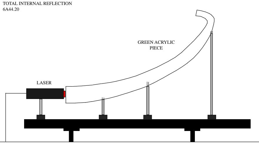
SET UP ON A LARGE OPTICAL BENCH ON A CART.
