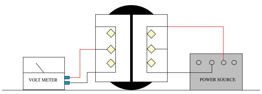
CONFIGURATION OF TRANSFORMER CAN BE CHANGED EITHER BY CHANGING WIRING POSITIONS OR BY CHANGING INSERTS.
