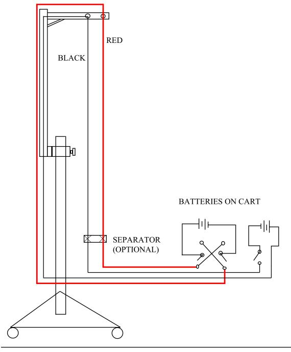
USE TRIANGLE BASE SET UP FOR MONKEY DROP. THE BASE IS ALREADY WIRED FOR THIS DEMO. DO NOT CHANGE WIRING.
