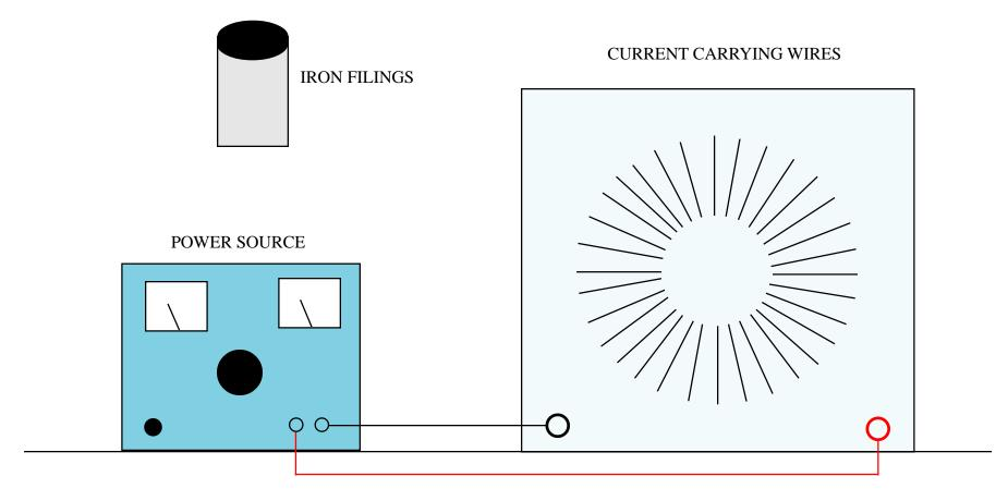
PLACE CURRENT CARRYING WIRE APPARATUS ON AN OVERHEAD PROJECTOR.
