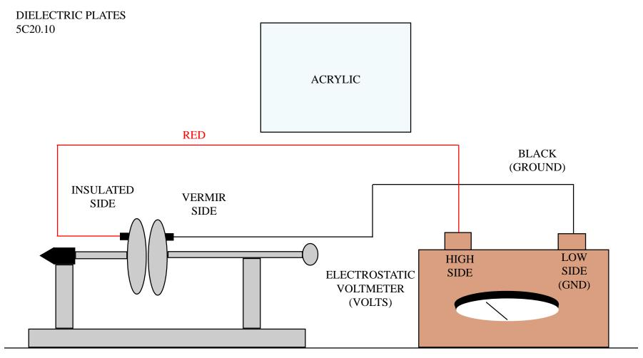
CHARGE WITH FUR AND PLASTIC ROD TO INSULATED SIDE. OR TRANSFER CHARGE FROM VDG
