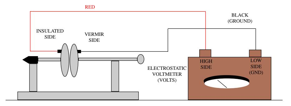
CHARGE WITH FUR AND PLASTIC ROD TO INSULATED SIDE. TRANSFER CHARGE FROM VDG
