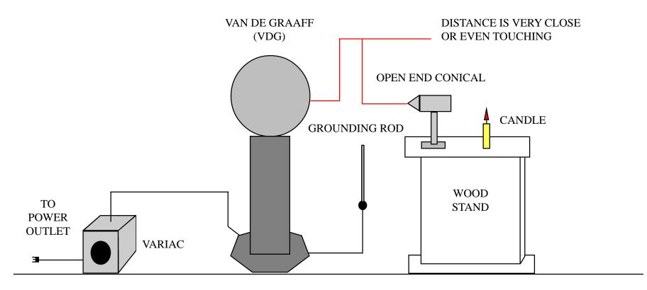
WHEN VDG IS IN OPERATION FLAME IS BLOWN "IN" TOWARD OPEN END CONICAL.
