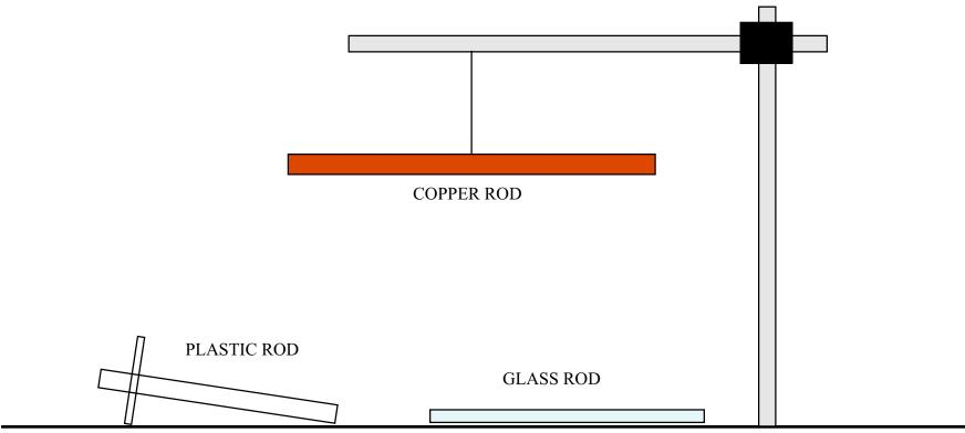
SUSPEND COPPER ROD FROM CROSS BAR BY FISHING LINE.
