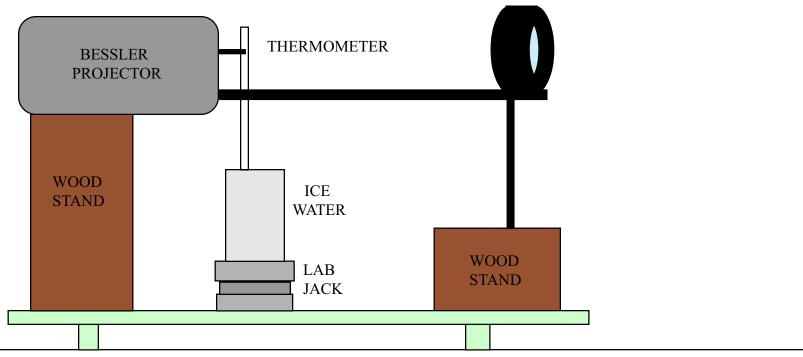
USE LARGE PROJECTOR THERMOMETER ATTACHMENT FOR BESSLER.
