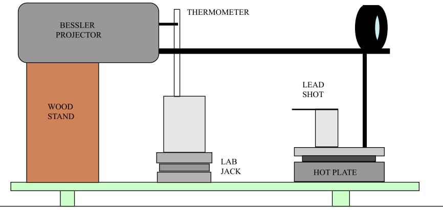
USE LARGE PROJECTOR THERMOMETER ATTACHMENT FOR BESSLER.
