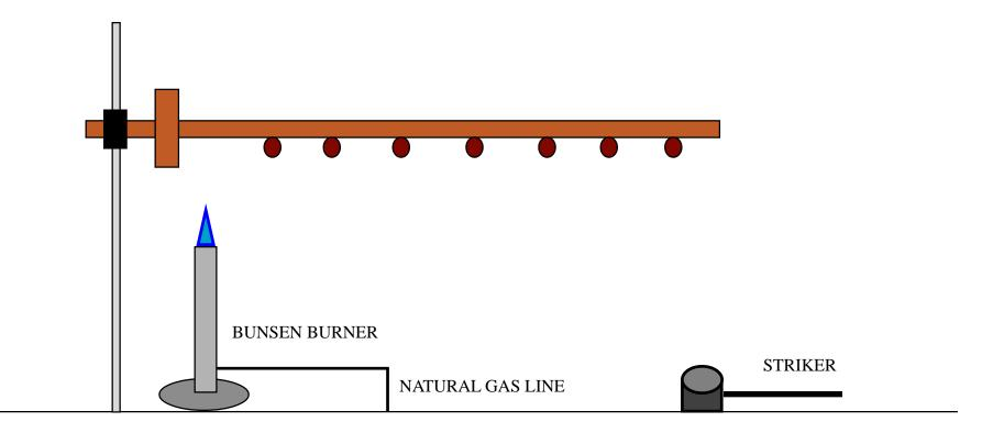
ATTACH STEEL BALL BEARINGS WITH CANDLE WAX.
