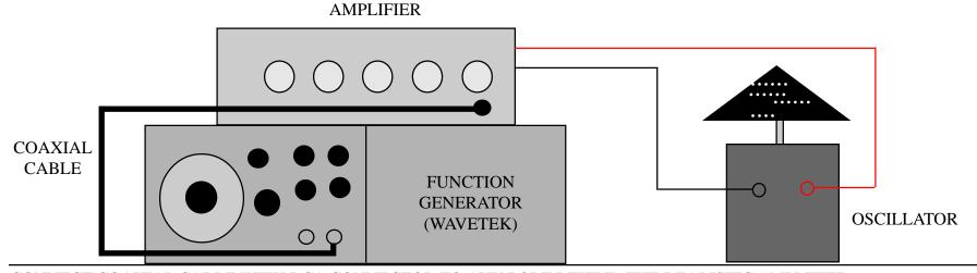
CONNECT COAXIAL CABLE WITH RCA CONNECTOR TO AUX PORT BEHIND THE REALISTIC AMPLIFIER.
