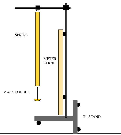
ATTACH METER STICK TO T - STAND WITH CLAMPS.
