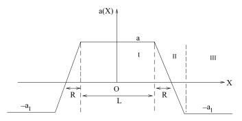
**Fig. 1.** The spatial dependence of the growth rate a(X) showing its value as the constant a in a segment of length L joined through a linear decrease to the value  $-a_1$  on both sides. The width of the transition region is R on either side.
