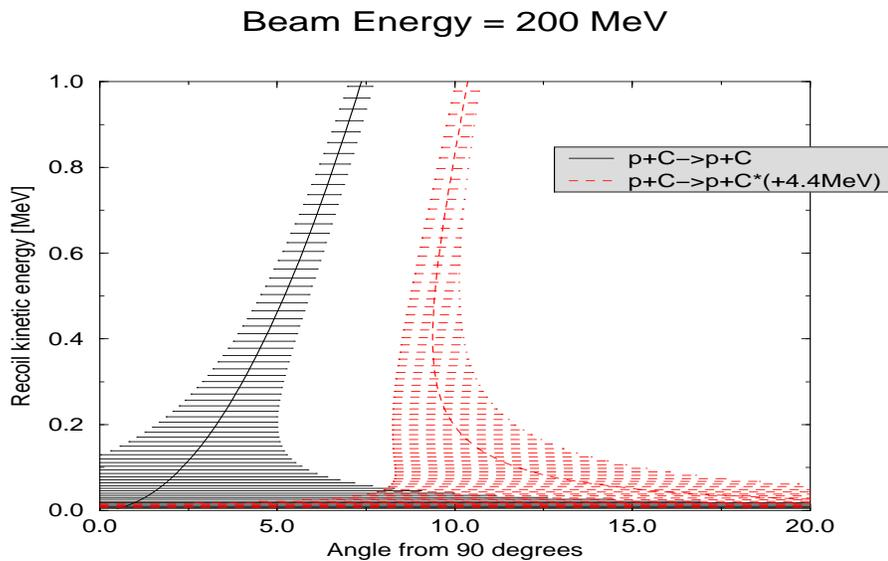
Figure 2. Energy-angle correlation for the elastic and inelastic recoil Carbon nucleus.
