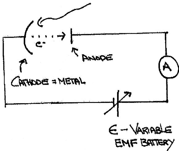
THE BATTERY ALLOWS US TO FIND THE C<sup>-</sup>'S KINETIC ENERGY. WHEN  $I = 0$ , WE SAY  $E = V_0$  = STOPPING POTENTIAL BECAUSE NO ELECTRONS ARE REACHING THE ANODE.
