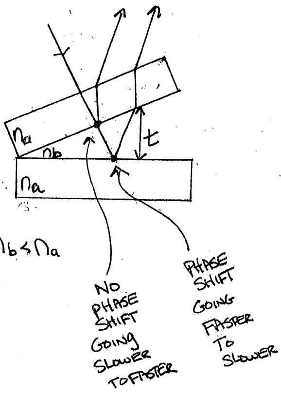
SO THE TWO BEAMS ARE ALREADY  $180^\circ$  OUT OF PHASE WHEN THEY INTERFERE  $\Rightarrow \vec{E}_p = \hat{e}(E_0)(\cos(Kz_1 - \omega t) - \cos(Kz_2 - \omega t))$
