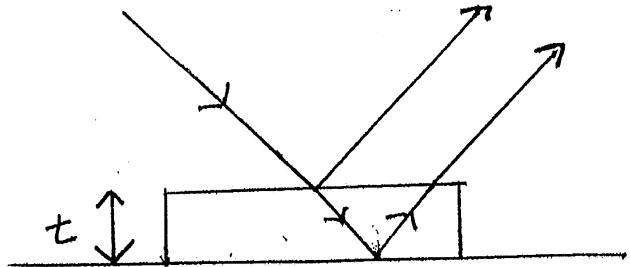
WHEN THE TWO BEAMS ARE BROUGHT TOGETHER (BY YOUR EYE USUALLY), THERE IS INTERFERENCE.
