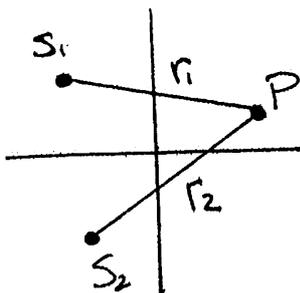
$$\text{CONSTRUCTIVE INTF.} \Rightarrow r_1 - r_2 = m\lambda$$
