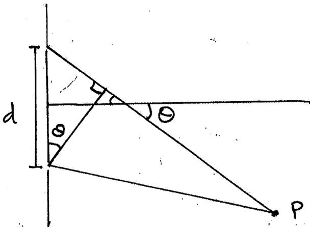
$\theta$  IS THE ANGLE FROM WHERE THE CENTER OF SLITS INTERCEPTS  $r$  TO THE POINT P.
