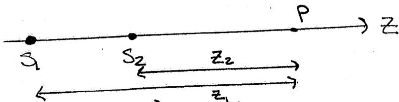
AT POINT P:  $\vec{E}_1 = \vec{E}_{01} \cos(k_1 z_1 - \omega_1 t)$ ,  $\vec{E}_2 = \vec{E}_{02} \cos(k_2 z_2 - \omega_2 t)$
