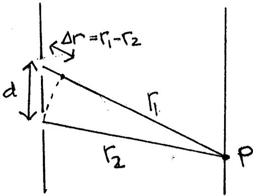
IF  $d$  IS VERY SMALL (IF THE SLITS ARE CLOSE TOGETHER) THEN THE ARC CONNECTING  $r_1$  AND  $r_2$  IS APPROXIMATELY A STRAIGHT LINE PERPENDICULAR TO  $r_2$
