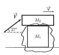
On the way to the recycling bin, he finds a box,  $M_2$ , of old physics demos, so he places it on top of the first. By exerting a force,  $\overrightarrow{\mathbf{F}}$  at 37° above the horizontal, to the upper box, he gets the combination to slide to the right.
