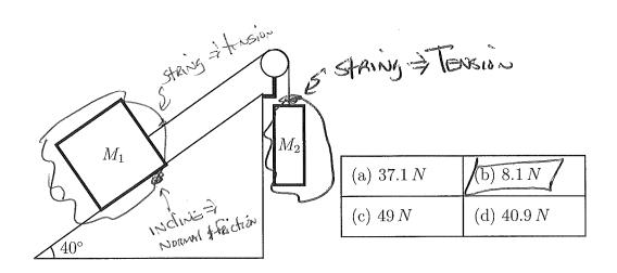
M<sub>1</sub> on incline =  $101 = M_1gsind = (6.5 kg)(9.8 m/s^2) sin 46 = 40.9N$  $W_1 = M_2gcosx = (6.5 kg)(9.8 m/s^2) cos 46 = 48.8N$
