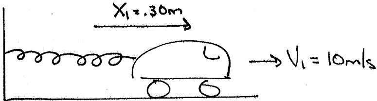
$$\text{MASS ON A SPRING} \Rightarrow X = A \cos(\omega t + \phi), V = -A\omega \sin(\omega t + \phi)$$
