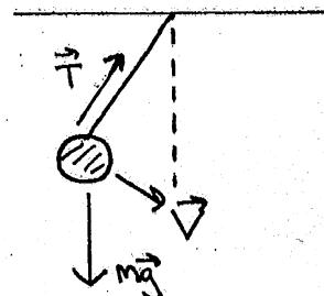
THE PENDULUM IS ALWAYS MOVING TOWARDS ITS EQUILIBRIUM POSITION BECAUSE OF THE RESTORING FORCE. IT DOESN'T STOP AT ITS EQUIL. POSITION BECAUSE OF ITS INERTIA.
