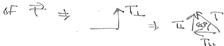
$$T_{\perp} = T \sin 60^{\circ} = T_A \left(\frac{\sqrt{3}}{2}\right) \Rightarrow \tau_{\perp} = \left(\frac{3L}{4}\right) T \left(\frac{\sqrt{3}}{2}\right)$$
