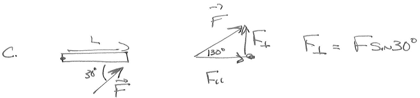
$$\tau = L F \sin 30^{\circ} = (4\text{m})(20\text{N}) \sin 30^{\circ} = 40\text{N}\cdot\text{m}$$
