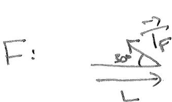
$$T = T_F L \sin 30^\circ = T_F L \left(\frac{1}{2}\right) \Rightarrow T_F = 2 \frac{T_{\text{sign}}}{L}$$
