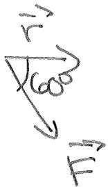
$$\tau = r F \sin \phi = (2\text{m})(20\text{N}) \sin 60^{\circ} = 34.64\text{N}\cdot\text{m}$$
