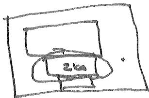
Forces on 2kg: Downwards force from 3kg  $\Rightarrow \vec{F}_{3\text{on}2}$  By 3<sup>rd</sup> Law  $\vec{F}_{3\text{on}2} = \vec{F}_{2\text{on}3}$
