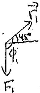
$$\tau_1 = r_1 F_1 \sin \phi = 0.09(\sqrt{2})(18) \sin(90^\circ + 45^\circ) \\ = 0.09(\sqrt{2})(18) \cos 45^\circ = 0.09(\sqrt{2})(18) \frac{1}{\sqrt{2}} \\ = (0.09)(18) = 1.62 \text{ N}\cdot\text{m}$$
