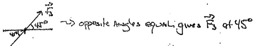
$$\tau_3 = r_3 F_3 \sin \phi_3 \quad \phi_3 = 45^\circ + 45^\circ = 90^\circ$$
