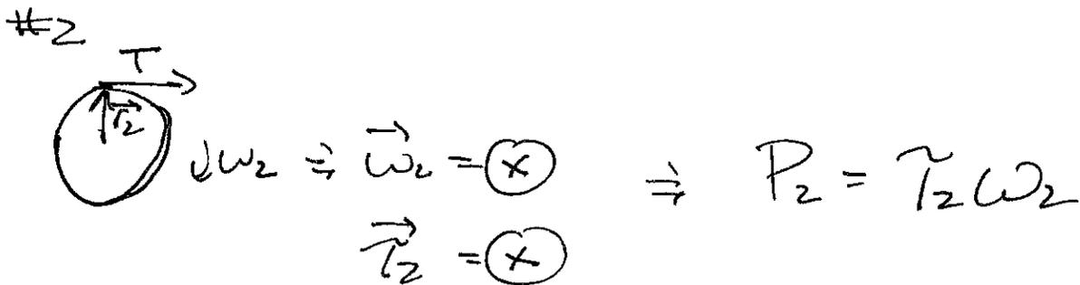
$$\Rightarrow \frac{P_1}{P_2} = \frac{\tau_1 \omega_1}{\tau_2 \omega_2} = \left( \frac{r_1}{r_2} \right) \left( \frac{\omega_1}{\omega_2} \right) = \left( \frac{r_1}{r_2} \right) \left( \frac{r_2}{r_1} \right) = 1$$
