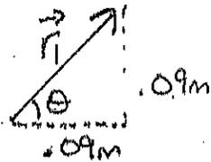
$$r_1 = \sqrt{(0.09\text{m})^2 + (0.09\text{m})^2} = 0.09(\sqrt{2})\text{m} \\ = 0.127\text{m}$$
