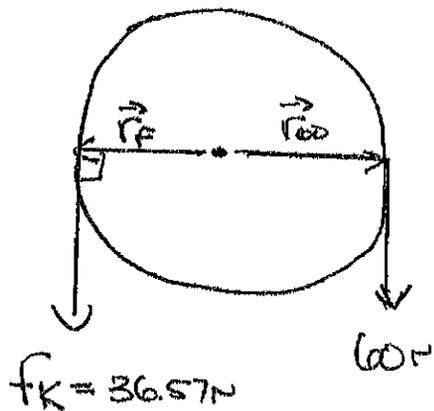
$$\begin{aligned} \vec{\tau}_F &= r_F f_K \sin 90^\circ, \odot \leftarrow \text{RHR} \\ &= R f_K, \odot \\ &= (.18\text{m})(36.57\text{N}), \odot \\ &= 6.5826\text{N}\cdot\text{m}, \odot \end{aligned}$$
