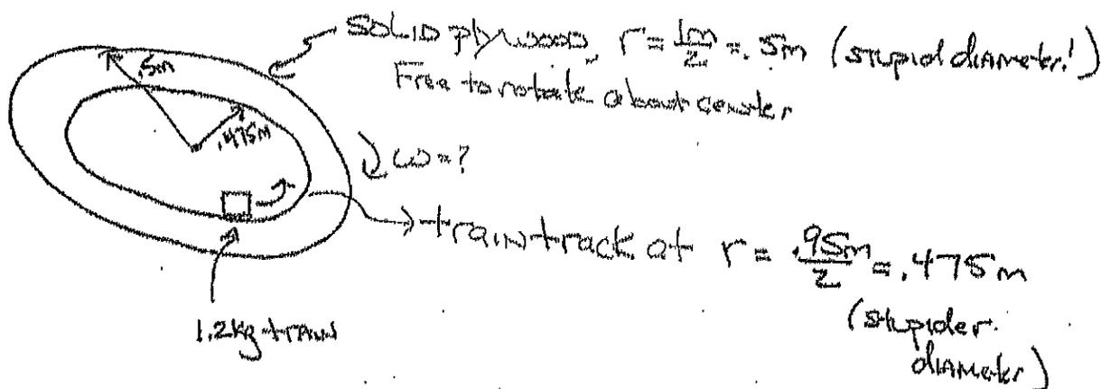
TRAIN AND PLYWOOD INITIALLY AT REST  $\Rightarrow L = 0$
