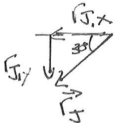
$$r_{J,x} = -r_J \cos 30^\circ = -16 \text{ m} \cos 30^\circ = -13.856 \text{ m}$$
