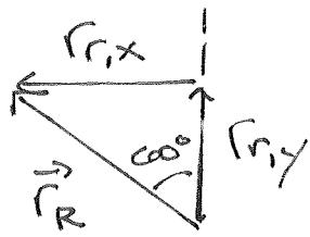
$$F_{r,x} = -F_r \sin 60^\circ = -26 \text{ m.s.} \sin 60^\circ = -22.5166 \text{ m}$$
