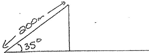
ROCKET ACCELERATED AT  $1.25 \text{ m/s}^2$  FOR 200M. THEN MOVES UNDER FORCE OF GRAVITY ONLY.
