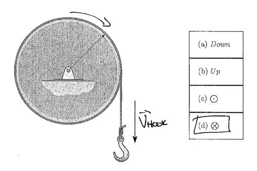
As Hook Falls, Drum spins clockwise RHR & B is into page = (x)
