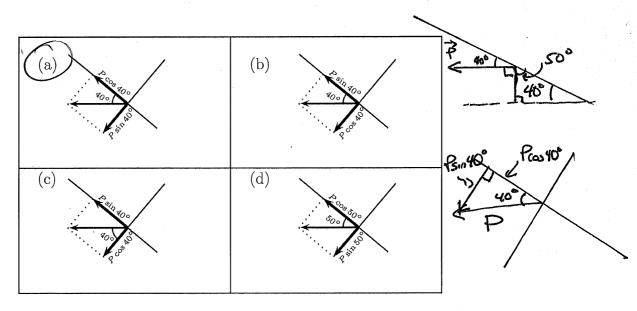
18. Which of the following is the correct listing of the parallel and perpendicular weight of the  $M = 1200 \, kg$  mass on the 40° incline? Note the use of kN = kiloNewtons to make the numbers smaller.
