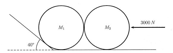
11. The instant Superman applies his horizontal force, which of the following is the correct free body diagram for  $M_2$ ? (Unlike Mastering Physics, I only care about direction!) In each case,  $n_{g2}$  is the normal force due to the ground while C is the normal force due to the contact between  $M_1$  and  $M_2$ .
