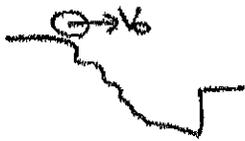
TO MISS PIT,  $x = 36\text{m}$  WHEN  $y = 25\text{m} - 45\text{m} = -20\text{m}$
