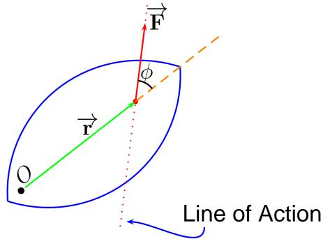
The calculation of torque can be simplified in some case by the use of the perpendicular distance.
