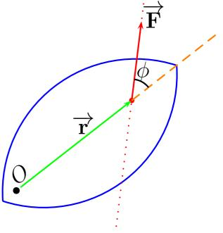
The calculation of torque can be simplified in some case by the use of the perpendicular distance.
