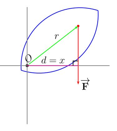
The perpendicular distance is particularly useful in finding the torque exerted by gravity (and any other vertical force).
