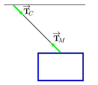
$\overrightarrow{\mathbf{T}}_{M} =$ force on mass due to bottom of rope
