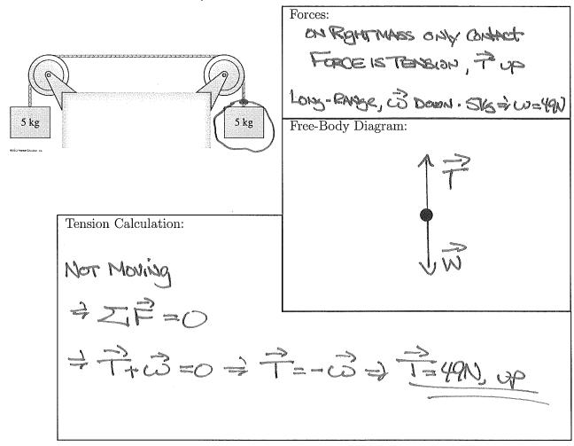
(c) Two 5 kg masses are connected to each over pulleys using a rope. What is the tension force that the rope exerts on the left-hand mass if they are both at rest?
