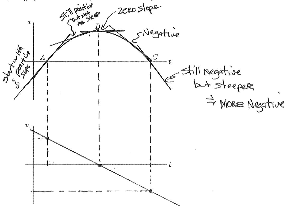
So: velocity begins positive <sup>at A</sup> AND goes down to zero at B. At C, it has become negative. Given the nice "symmetry" of the curve, the velocity at C is same magnitude as velocity at A. Connecting dots, we find velocity is a straight line
