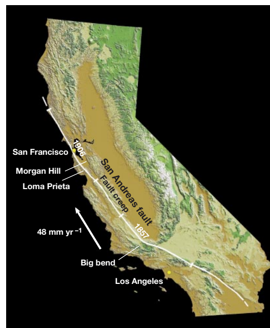
Figure 1 The San Andreas fault. The fault marks the divide between the Pacific and North American tectonic plates, and accommodates about 35 mm of the annual 48 mm of relative motion between them. The northern and southern segments last broke in major earthquakes in 1906 (magnitude 7.8) and 1857 (magnitude 8.2), respectively; the central section creeps steadily and does not accumulate strain. The other places marked are cited in the text. The physics of faulting is poorly understood, and the question of whether the San Andreas is a weak fault in a strong crust, or a strong fault in a strong crust (as Scholz 2 proposes), remains controversial. (Courtesy of the US Geological Survey.)
